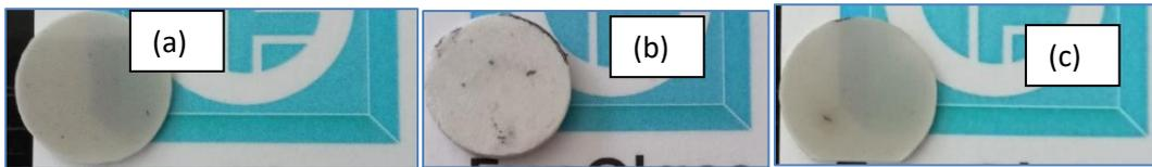
Fig. 2: The photograph of the prepared translucent YAG glass/ceramic with diameter 12 mm placed on the text. Pressure used during densification a) 60 MPa; b) 70 MPa; c) 80 MPa.
