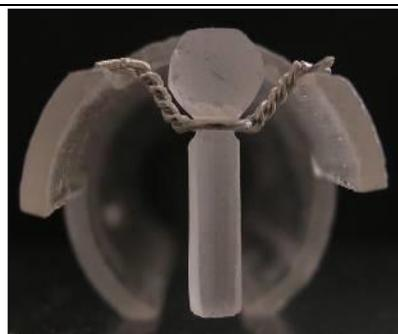
Figure 2: Sample prepared for the measurement by the pendant drop method.
