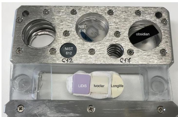
Figure 2 sample holder with analyzed samples
