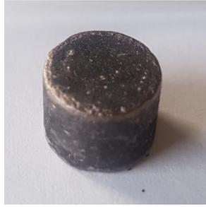
Fig.5. YB<sub>4</sub> sample after oxidation at 1400 °C for 1 hour: a) before spallation, b) after spallation
